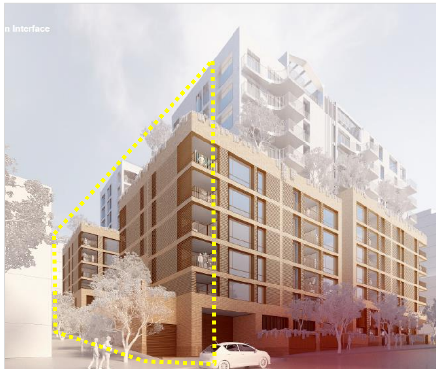
Figure 5: Graphic representation demonstrating narrow windows, screening, and materiality of southern elevation (Source: Silvester Fuller)
